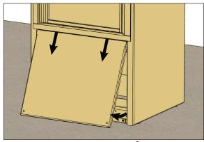
**D.** Remove and discard the plastic push-in rivets which hold the two mounting brackets and two skirt plates in place inside the lower compartment of the PORT cabinet.
