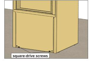
2). Pull the panel out at the bottom and down from behind the PORT package-box trim.
