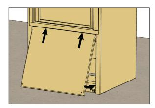
**B.** Secure the lower-front panel to the cabinet using a #2 square-tip 1/4" hex-shank insert driver bit and the two (2) screws removed at the start of the installation.
